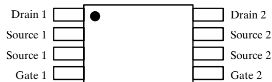
Figure 3. Pinouts for Dual-Die LITE FOOT
